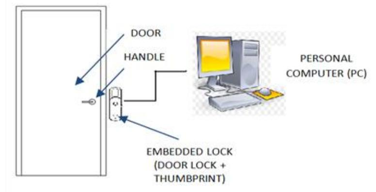
**Figure 1 : Embedded Door Lock System using Biometric Technology**
