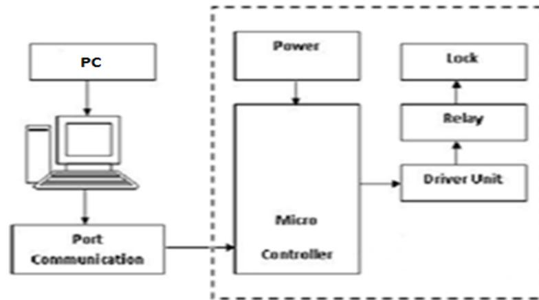
**Figure 2. Diagram of Embedded Door Lock System**
