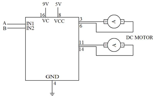
**Figure 11: A Simple Schematic for Interfacing a Dc Motor Using L293d**
