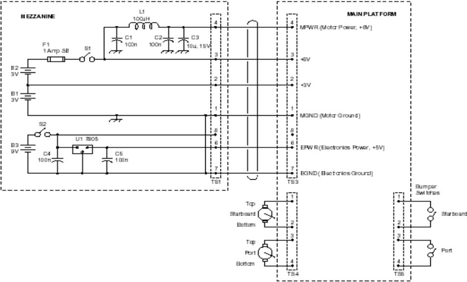
**Figure 3: Power Wiring**
