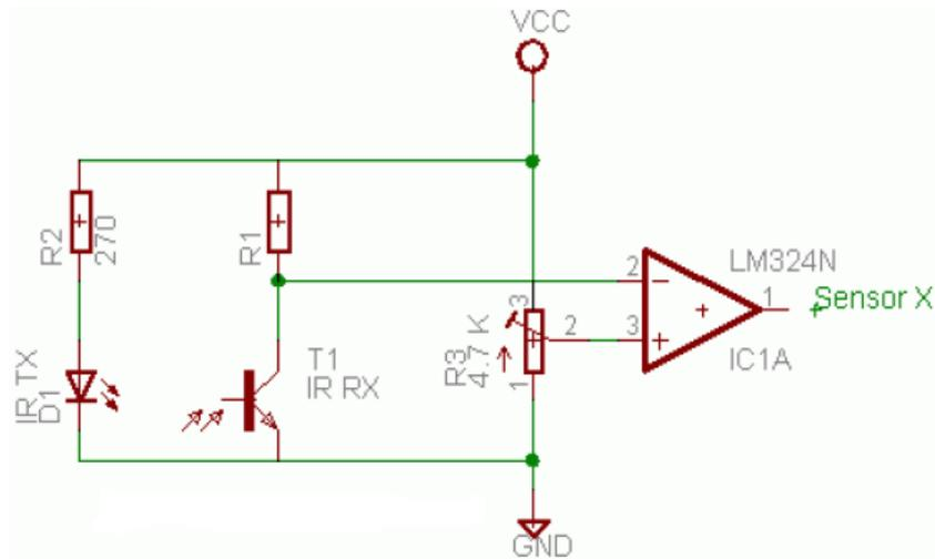
**Figure 6: Schematic of Single Sensor**
