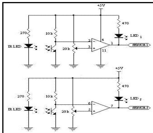
**Figure 8: Sensor Circuit**
