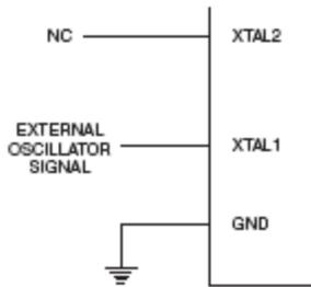
**Figure 13: External Clock Drive Configuration**
