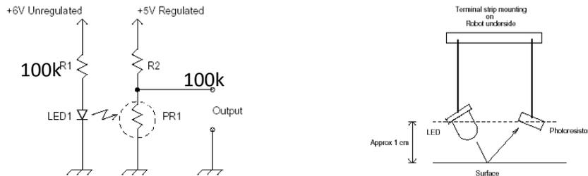
**Figure 1: Photodetector Circuit**
