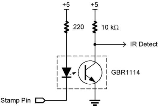
**Figure 4: IR emitter/detector**
