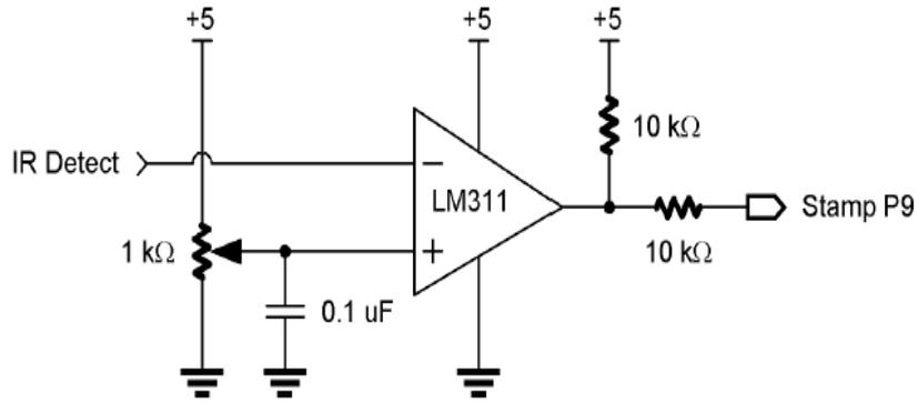
**Figure 5: Threshold Comparator Circuit**
