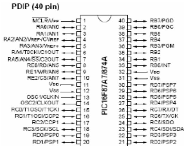
**Figure 3: PIC 16F877A Microcontroller**
