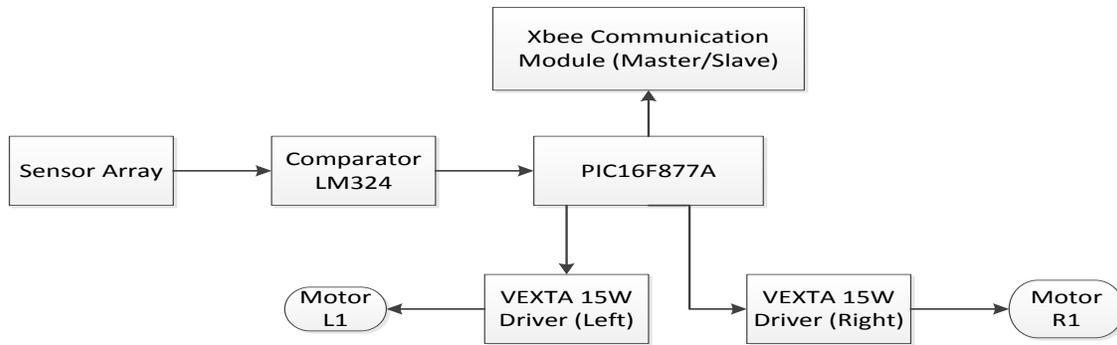
**Figure 2: Block Diagram of Development of Controller System**
