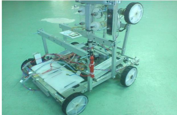
**Figure 4: Automatic Guided Vehicle (KOGAS 1)**
