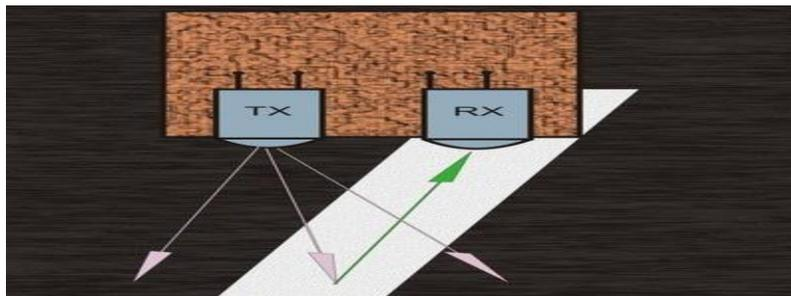
**Figure 5: Infrared Reflection (Source : S.F.Mansour, 2011)**
