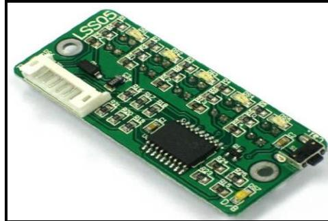
**Figure 5: Auto Calibrating Line Sensor**
