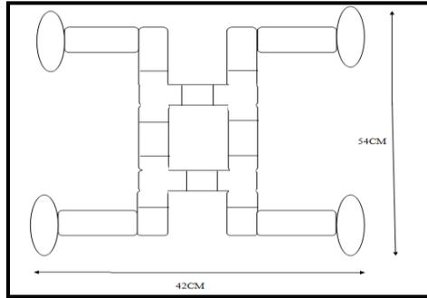
**Figure 8: Top View of the Robot**
